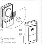
(3) Hole for removing the case (When replacing the battery, use a screwdriver to carefully separate the case through this hole)
